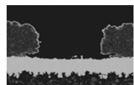
Electless copper plating (40µm)
