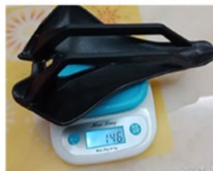
One piece saddle of recycled carbon fiber composite
