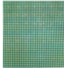
Molded Body of SHF and PCB (Before Thermal Cycle Test)
