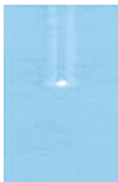
▲圖八 Streak Line 塗佈缺陷
